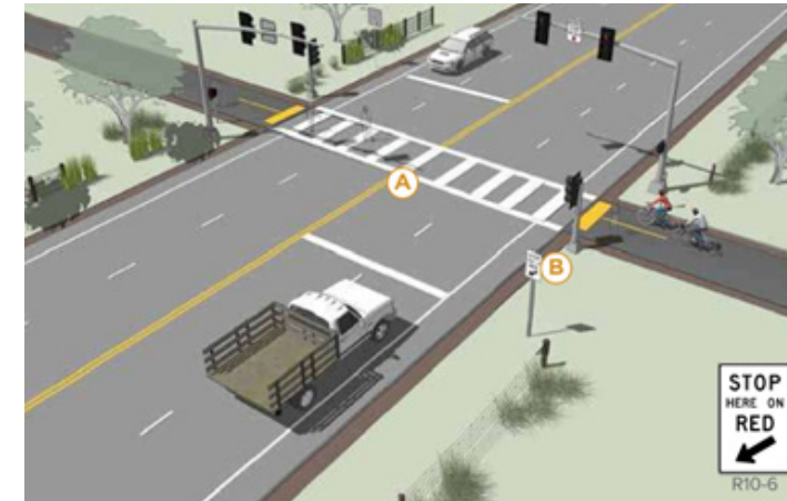
Full Traffic Signal Crossing, 2017 Empire State Trail Design Guide, page 5-56.
