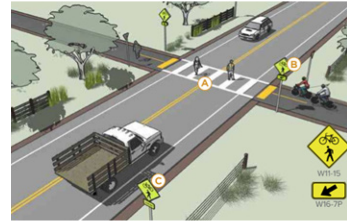
Marked and Signed Crosswalk, 2017 Empire State Trail Design Guide, page 5-44.
