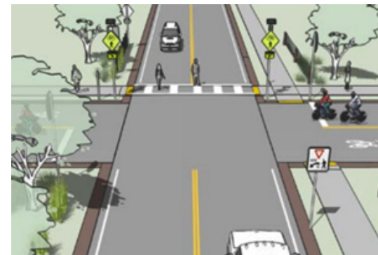
At-grade Road Crossing with Signage.
